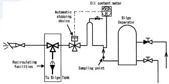
Figure 1.1 Oily-water Separating Equipment
