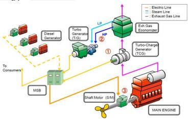
Figure 1.15 Rankine Cycle Generator
