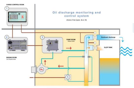
Figure 1.2 Oil Discharge Monitoring and Control System (Courtesy of HSN-KIKAI KOGYO Co., Ltd.)
