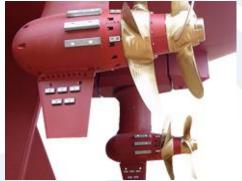
Figure 1.17 Contra-rotating Propeller (Courtesy of Nakashima Propeller Co., Ltd.)
