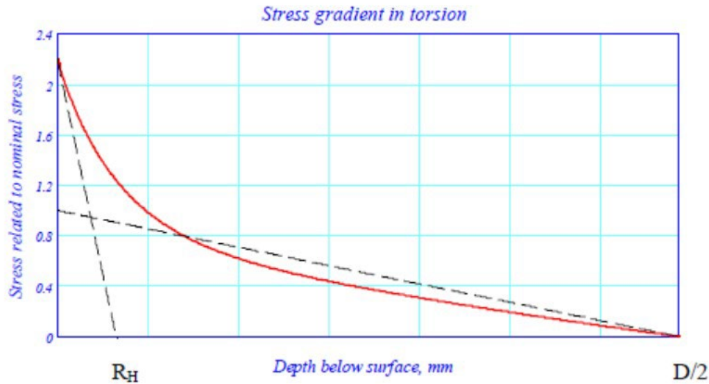
Figure 3.3. Torsional SCF in the crankpin fillet as a function of depth. The corresponding SCF for the journal fillet can be found by replacing R_H with R_G and D with D_G
