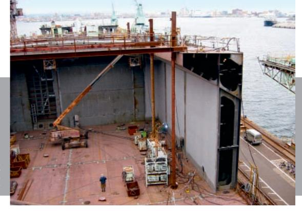
A double side skin bulk carrier under construction at Hakodate Dock
