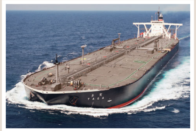
TAGA A 303,430 dwt oil carrier built by Universal Shipbuilding Corporation for Blue Tree Maritima S.A.
