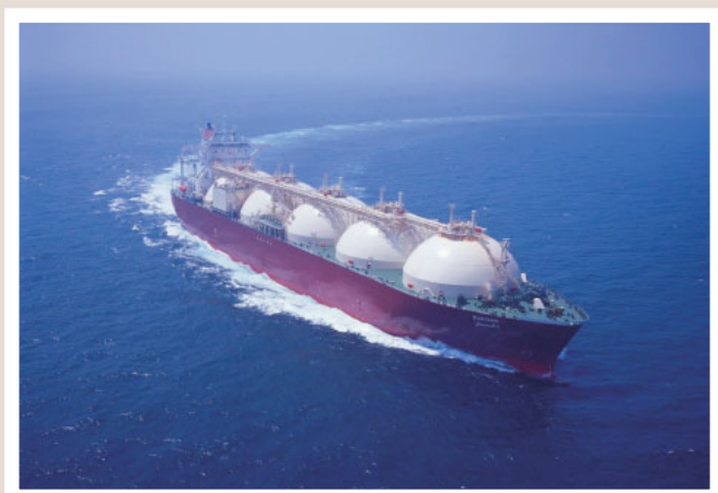
DUKHAN A 137,661m 3 LNG Carrier built by Mitsui Engineering & Shipbuilding Co., Ltd., for Qatar LNG Transport Limited.
