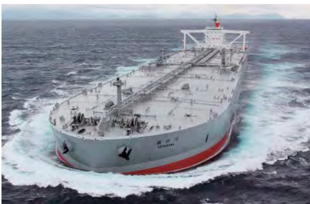
SETAGAWA a 299,998 dwt oil carrier built by IHI Marine United Inc., Kure Shipyard for Kawasaki Kisen Kaisha, Ltd.
