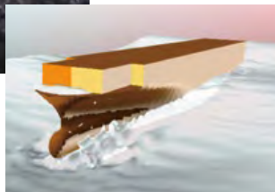
Top: Towing tank test of the response of large container ships to whipping Bottom: Computer simulation of the response of large container ships to high waves
