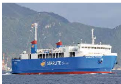
STARLITE PIONEER 2,682gt PASSENGER/RO-RO CARGO SHIP built by KEGOYA DOCK CO., LTD. for STARLITE FERRIES, INC.
