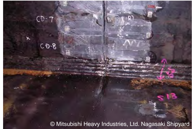
Large scale crack arrest test (Crack arrest design)
