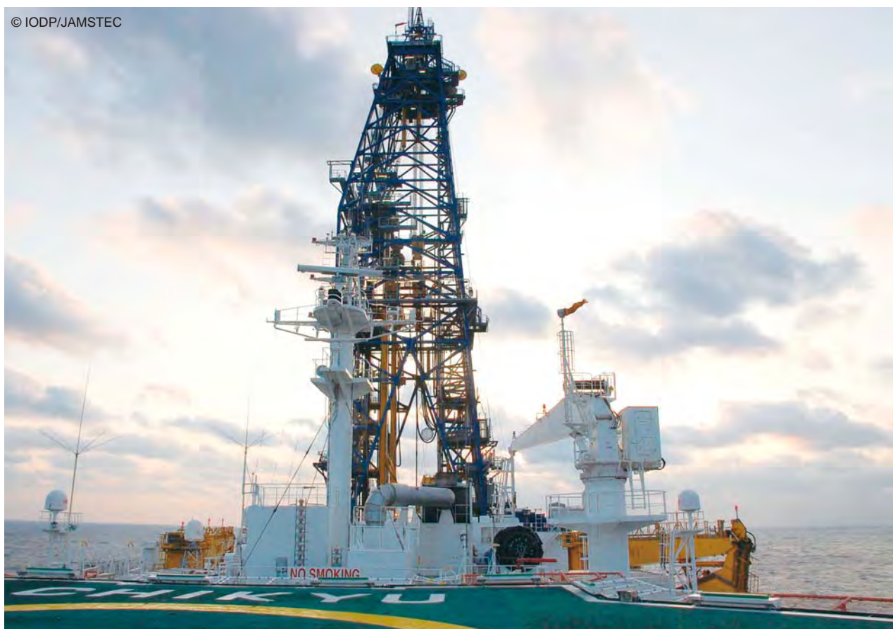
The Chikyu 's riser drilling system
