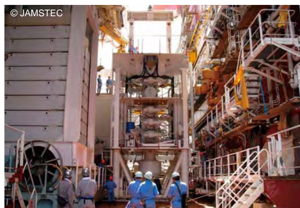
The blow-out preventer is an essential part of the riser system.
