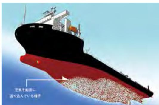
Air lubrication system for reducing frictional resistance between vessel bottom and water
