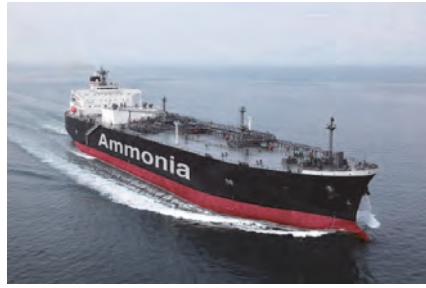
Fig. 2 Ammonia-fueled ammonia transport ship
