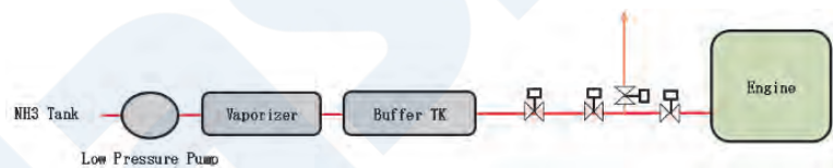
Fig. 4 Fuel supply system for four-stroke engine
