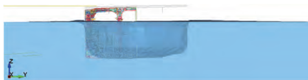
Fig. 6 Sway motion of the struck ship and disturbed fluid surface obtained by NLFEA with S-ALE at final time of simulation. Surge velocity of the striking ship is 6 kt.
