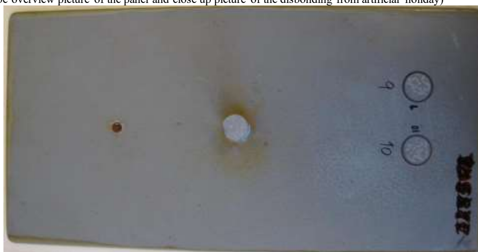
Figure C-1 Disbonding from artificial holiday, bottom wave tank panel (example picture not connected to example results in this model report).
