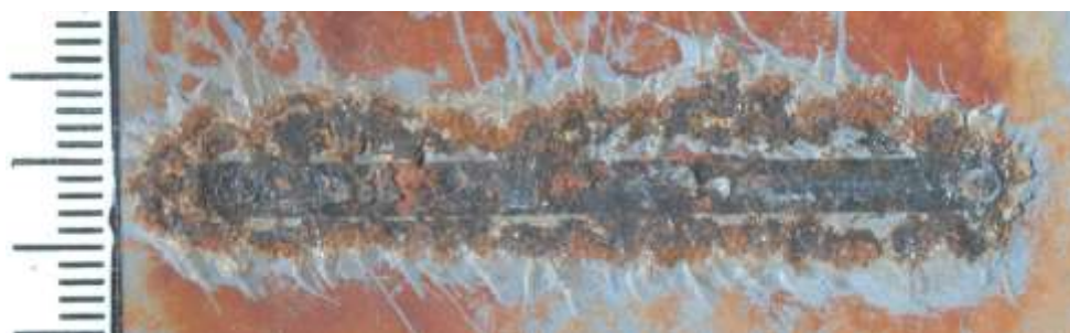
Figure C-4 Undercutting from scribe, top wave tank panel (example picture not connected to example results in this model report).
