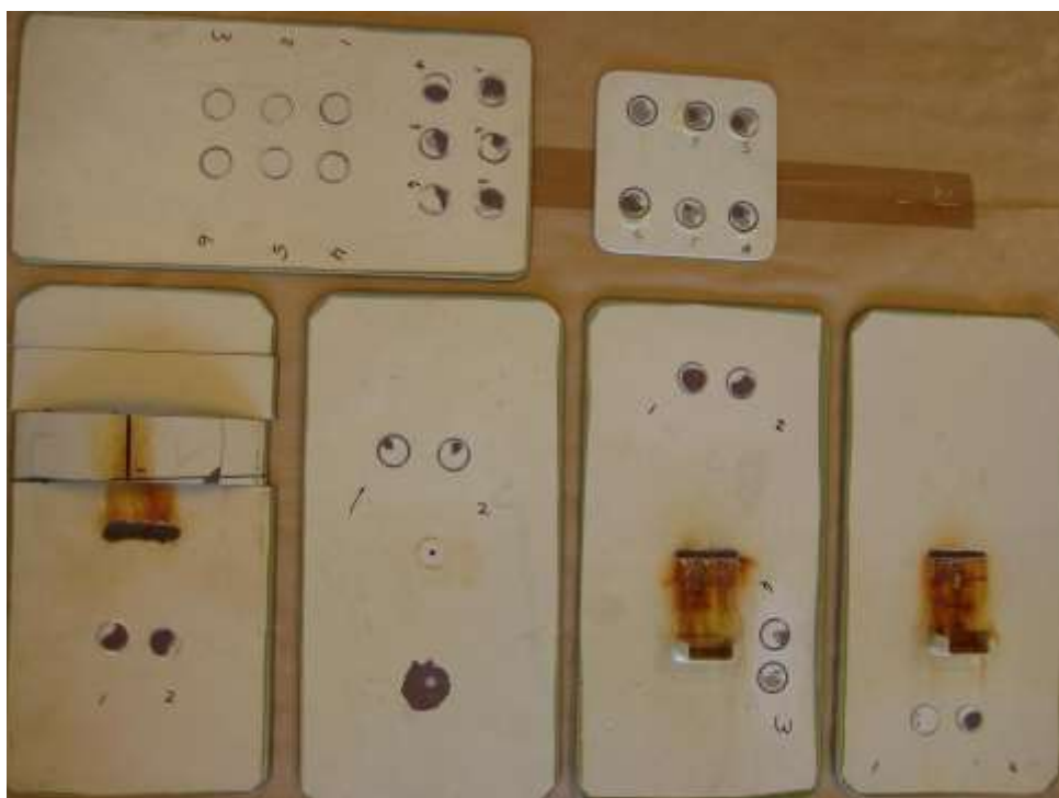
Figure C-1 Overview picture of the panels after exposure in the wave tank and the heating chamber. Reference panel not exposed on the top right. Picture taken after examination (example picture not connected to example results in this model report).
