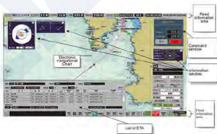
Figure 3 Automatic Maneuvering System
