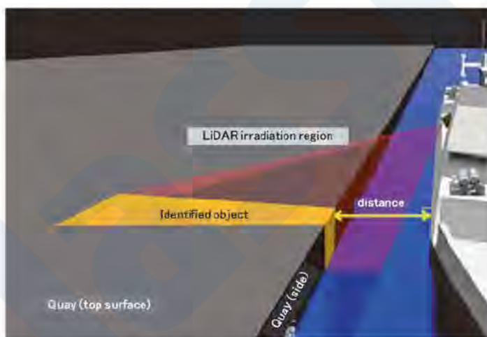
Figure 6 Outline of Quay Ranging System
