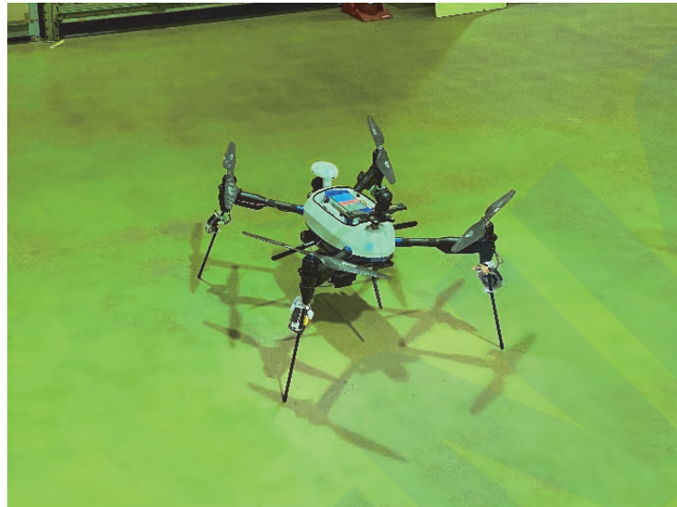
Photo 2 Autonomous drone equipped with vision sensor
