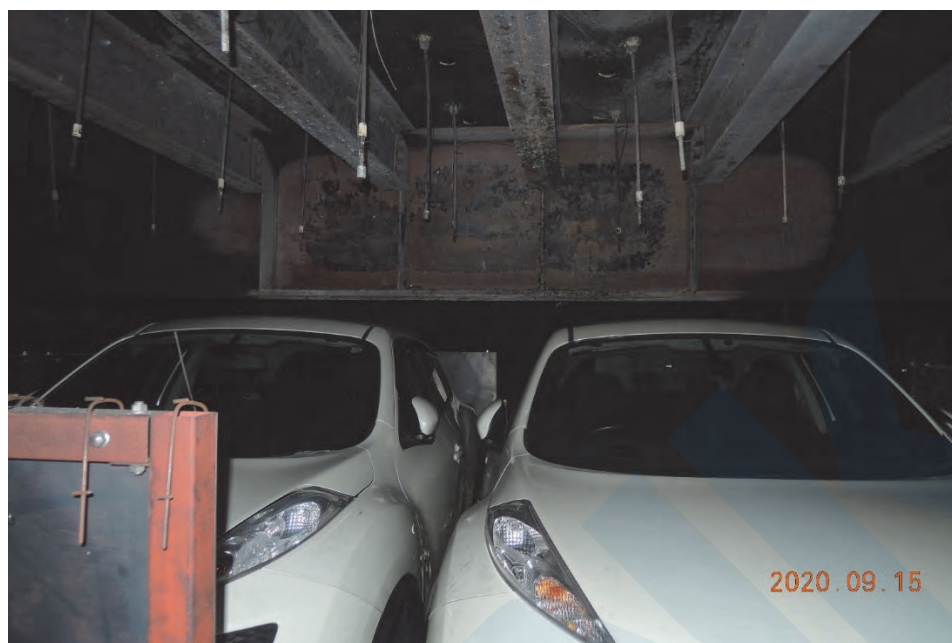
Figure 5 Photograph of a vehicle fire experiment: Condition of horizontal arrangement
