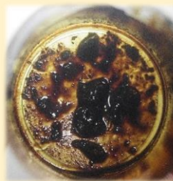
Image2 Sludge formation in poor compatibility of VLSFO (flocculated sludge is formed and deposited at the bottom)
