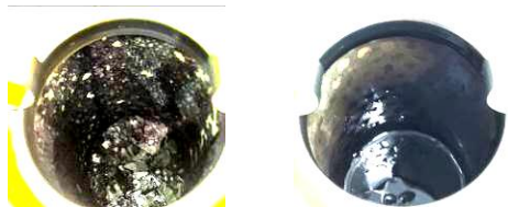
Fig 6. Test engine strainer condition Left: ExtRS not added Right: ExtRS 10% added
