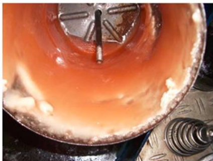
Filter blocked due to wax deposit Source: 01|2015 CIMAC Guideline
