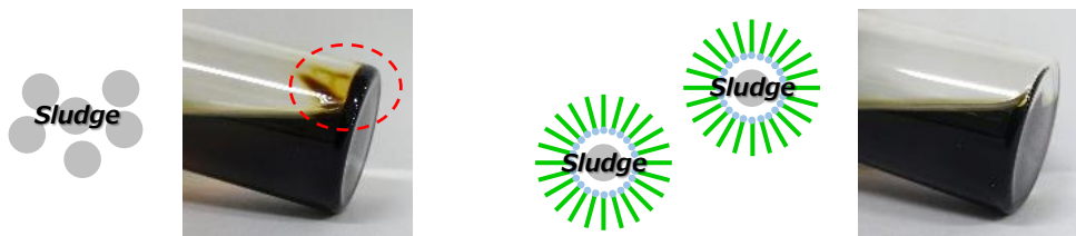
Figure 4. Image of sludge dispersion by SD-20
