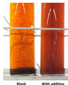
Fig. 3. Dispersion test with n-heptane.
