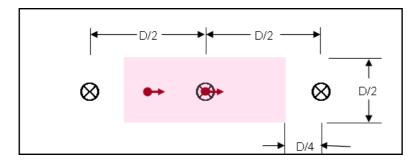
For this system, the outer nozzles should be placed outside of the protected area a distance of at least 1/4 of the maximum nozzle spacing.
