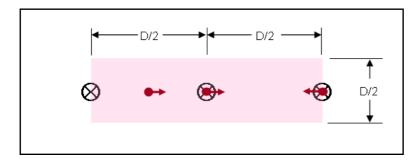
For this system, outer nozzles should be placed at least at the edge of the protected area.
