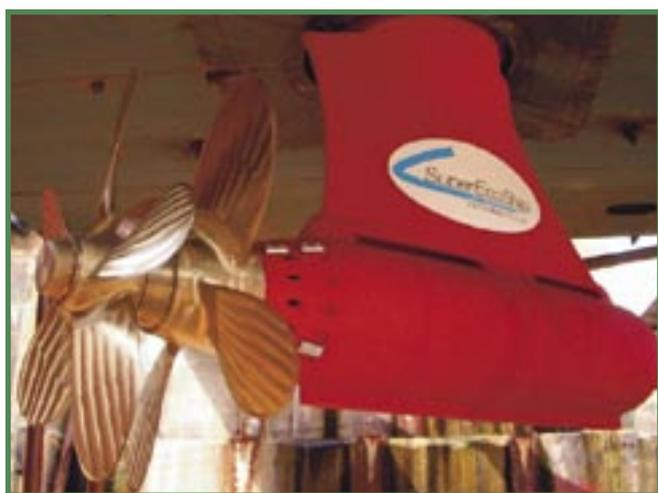
Fig. 2 Full-scale model of contra-rotating pod propellers for test use
