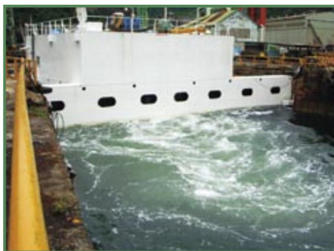
Fig. 3 View of testing of full-scale model of contra-rotating pod propellers
