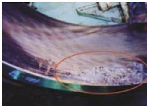
Fig. 1 Bearing damage
