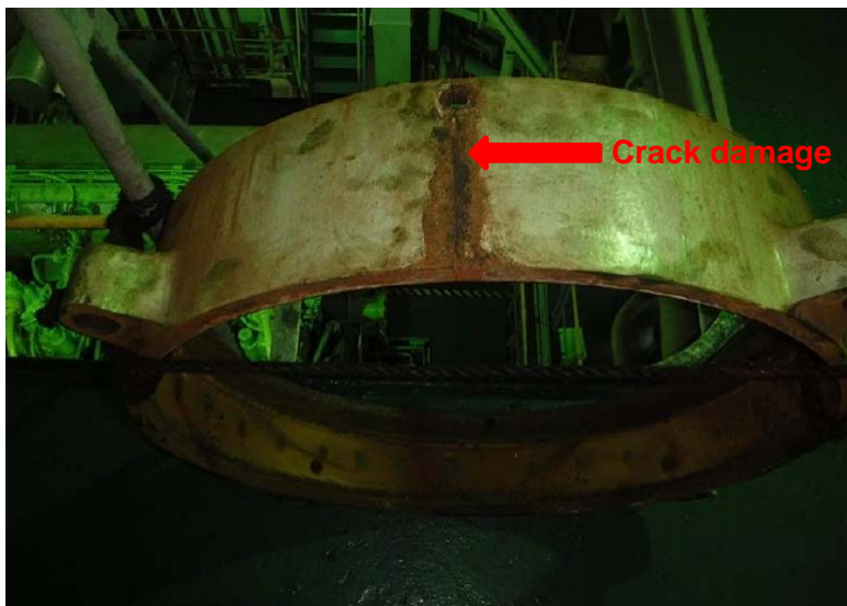
Photo 1 Crack damage on cooling jacket, initiated from bolt hole in many cases.
