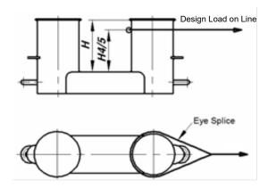
3.5.3 Under the design load conditions as specified in 3.3 the allowable normal stress should be taken as 100% and the allowable shearing stress as 60% of the specified yield point for the material used. Normal stress is the sum of bending stress and axial stress with the corresponding shearing stress acting perpendicular to the normal stress. No stress concentration factors being taken into account.
