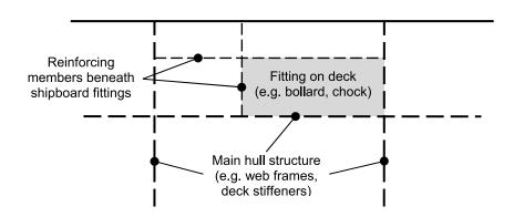
The acting point of the towing force on shipboard fittings is to be taken at the attachment point of a towing line or at a change in its direction. For bollards and bitts the attachment point of the towing line is to be taken not less than 4/5 of the tube height above the base, see figure below.
