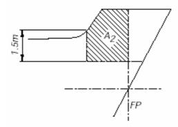
The equipment length of the ships is the length between perpendiculars but should not be less than 96% nor greater than 97% of the extreme length on the Summer Waterline (measured from the forward end of the waterline).
