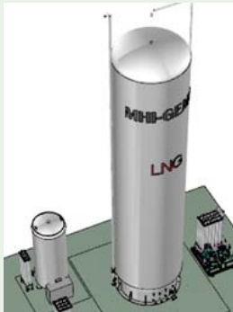
Storage / Double wall tank
