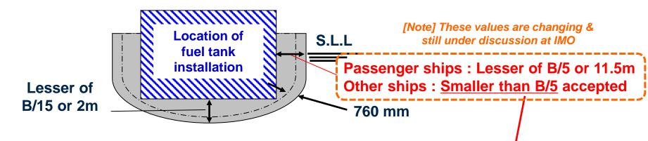
ClassNK "Guidelines for Gas Fuelled Ships" = "d" in New IGC Code 2.4
