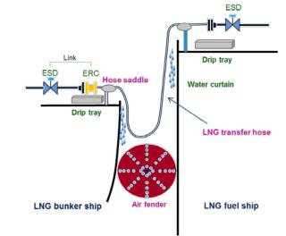
Arrangement of LNG bunkering equipment (example of STS)
