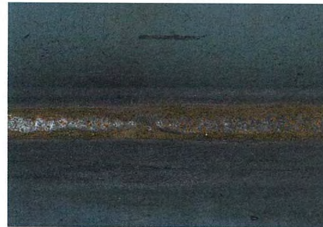
C1.3 Automatic fillet weld
