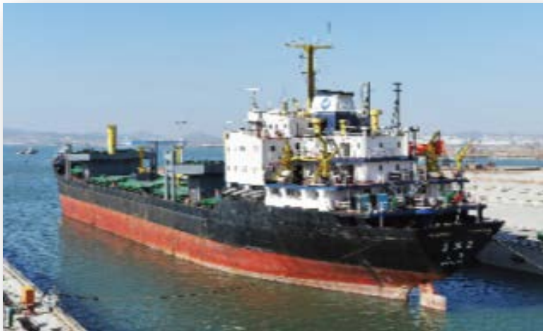
MV SHENHAI 2 Owner: China Shipping Type: B/C DWT: 9,874 tons LDT: 5419 Long ton
