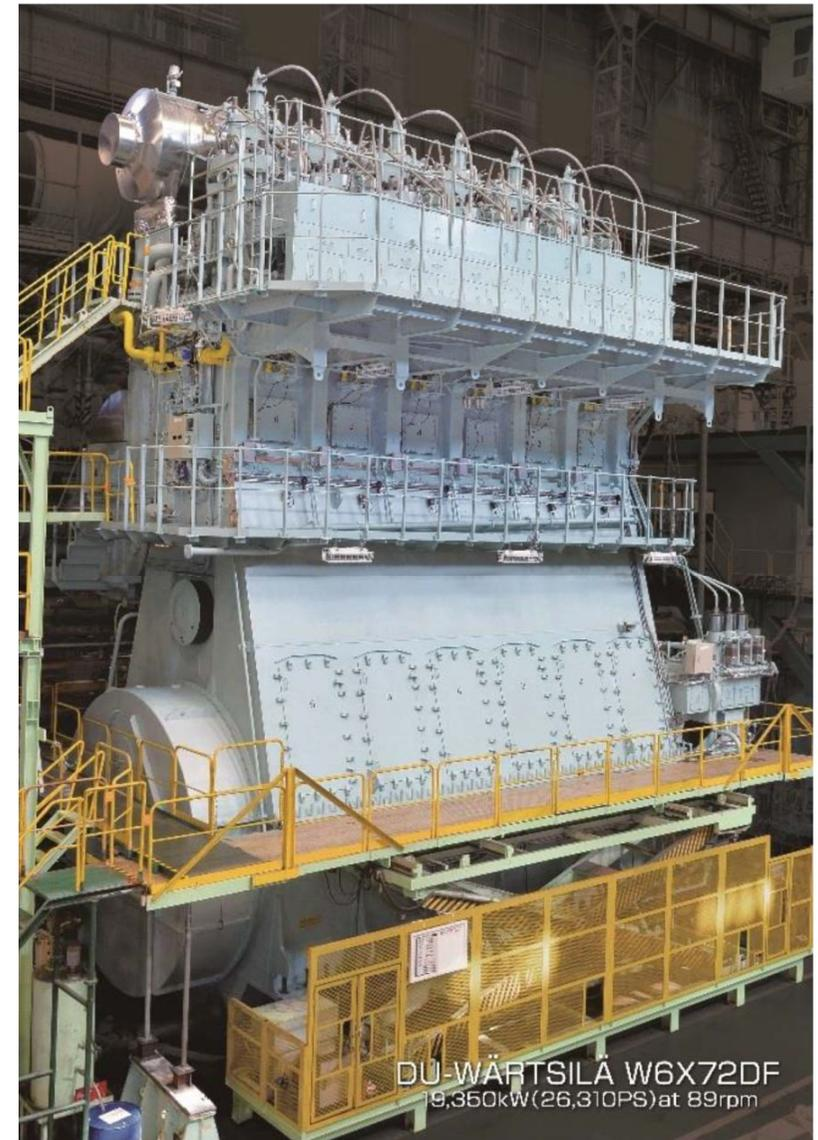
Figure1 Test engine (W6X72DF)
