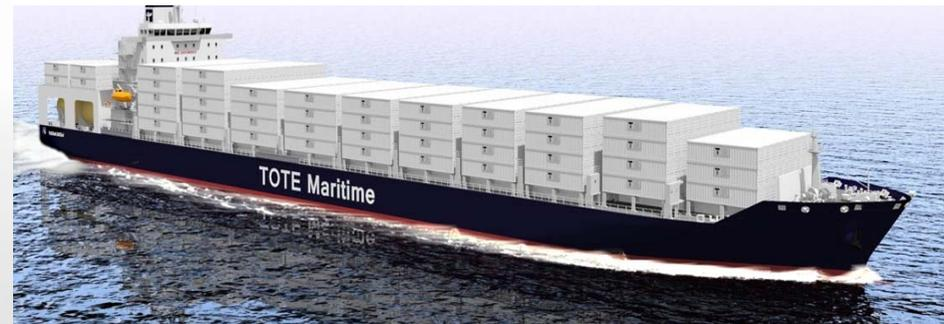
• TOTE Line has ordered 3,100TEU container ships propelled by MAN low-speed ME-GI gas (DF) engine. (Route: Florida⇔ Puerto Rico)
