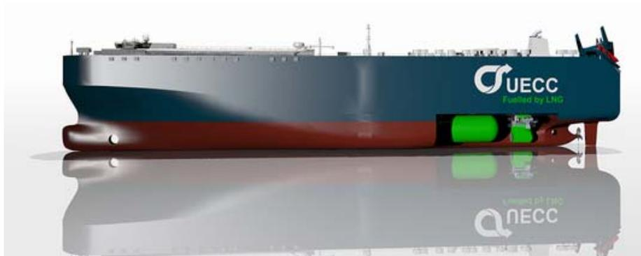
• United European Car Carriers (UECC) jointly owned by NYK and Wallenius Lines has ordered KHI two PCCs propelled by MAN low-speed ME-GI gas (DF) engine. (for voyage in European ECA)
