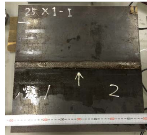
板厚25mm, 溶接線長約400mm(X開先)
