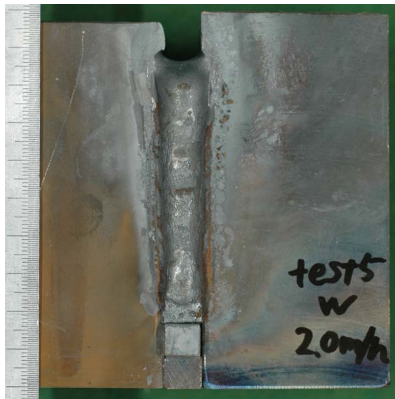
Welding speed : 2m/h
