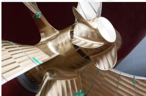
Figure 1.18 Propeller Boss Cap Fins (PBCF) (Courtesy of MOL Techno-Trade, Ltd.)
