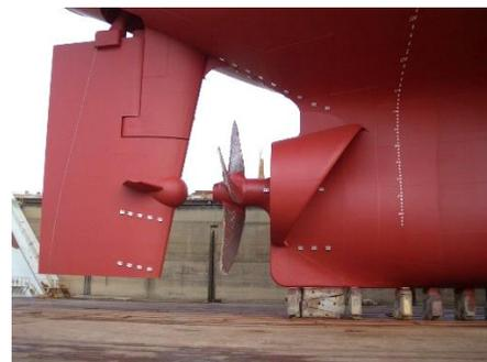
Figure 1.19 SURF-BULB (Courtesy of Japan Marine United Corporation)
