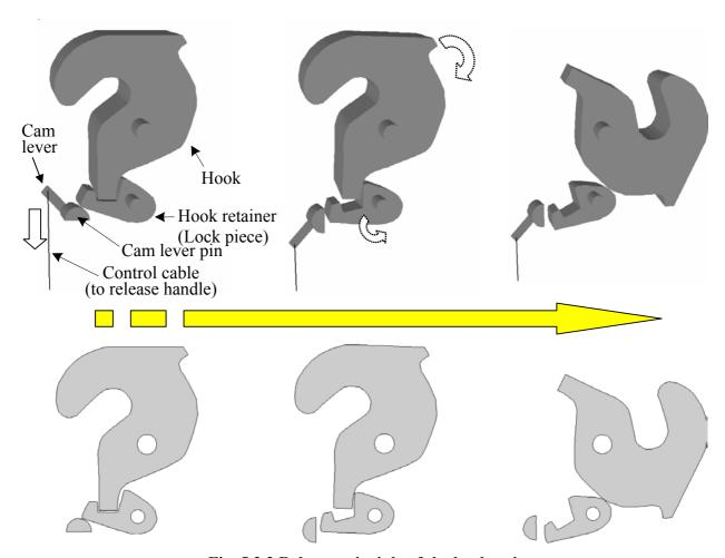
Fig. 5.2.2 Release principle of the hook unit
