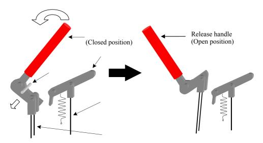
Fig. 5.3.2 Operation procedure of the release handle
