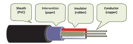
**Figure 2 –** Example of homogeneous materials (cable)
