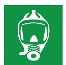
The location and the number of EEBDs shall be indicated in the fire control plan [Reg 13.4.3.2]. The relevant drawing should be endorsed by the attending surveyor after confirming the provision of EEBDs are in accordance with the regulations. The symbol for EEBD (see *left*) from the International Standard ISO 17631 *Ships and marine technology* – *Shipboard plans for fire protection, life-saving appliances, and means of escape* may be used, as IMO
