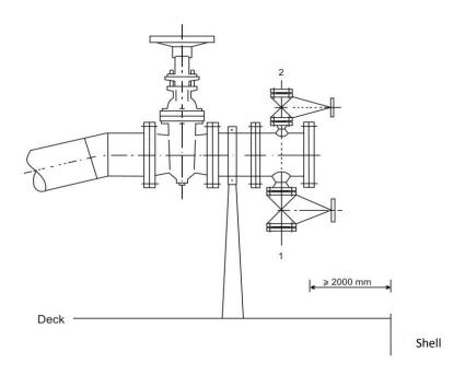
Connection for discharging residues. Connection pursuant to standards:
