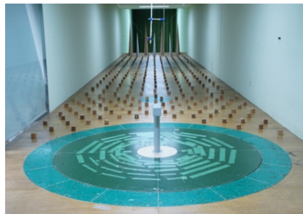
b) Installation of turbulent boundary layer generator
