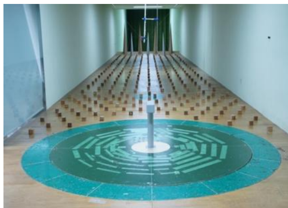
b) Installation of turbulent boundary layer generator
