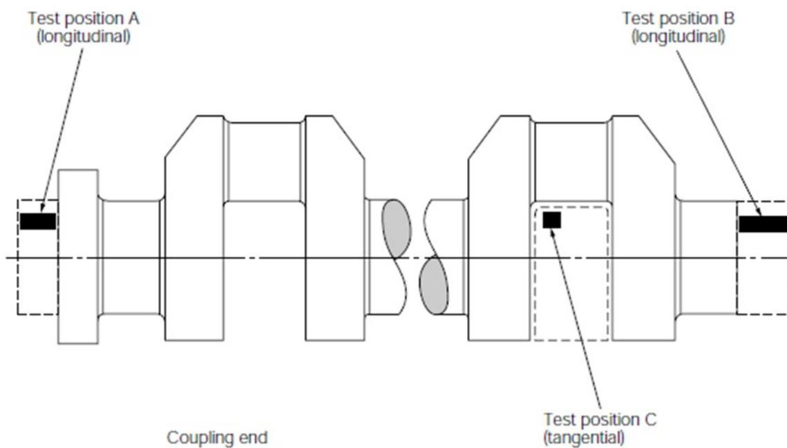
Fig. 98 Solid forged crankshaft
