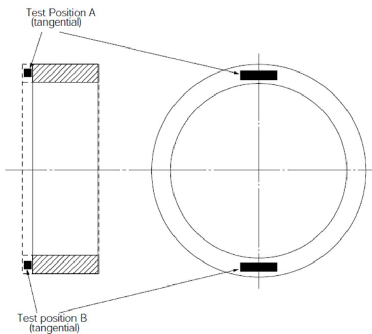
**Fig. 76** Gear rim (made by expanding)
