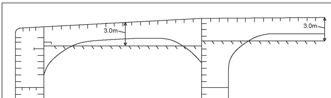
**Figure 4 Maximum water level in a tank**
