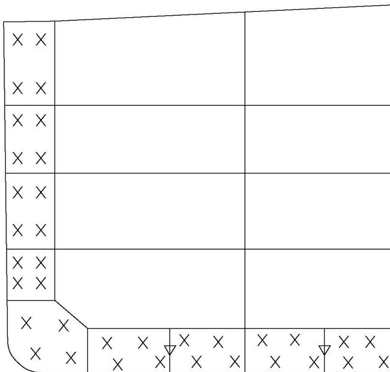
**Figure 8 - Transverse bulkheads in ballast tanks**
