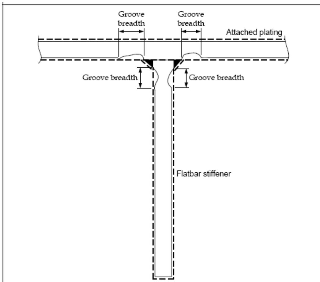
**Figure 3 - Grooving corrosion**
