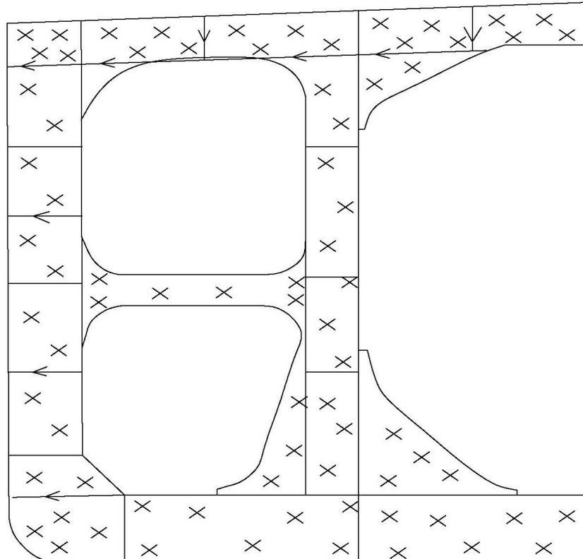
**Figure 6 - Transverse rings in cargo and ballast tanks**
