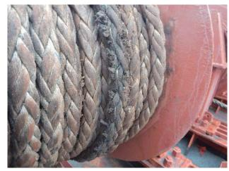
Deteriorated mooring ropes
