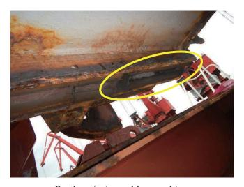
Partly missing rubber packing
