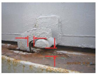
Excessive gaps of hatch cover
