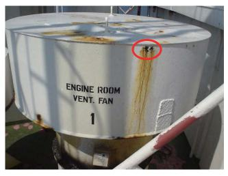
Corrosion holes in the casing of ventilator
