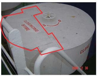
Inappropriate temporary repair by tape
