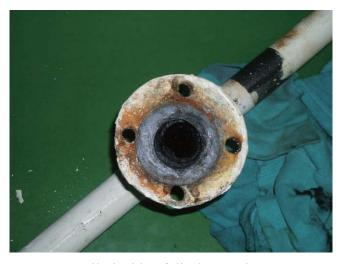
Oily inside of discharge pipe
