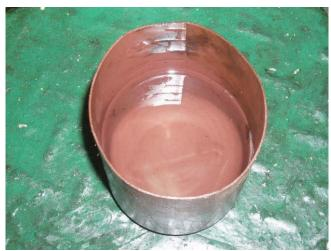
Clean sampling water (after flushing)
