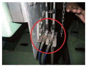
Bent release cable and bracket
