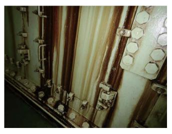
Oil leakage of M/E
