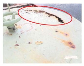
Corrosion holes in the casing of ventilator
