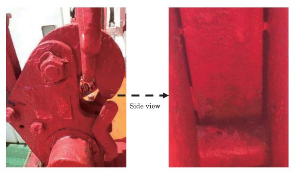
Seize of on-load release gear by excessive paint
