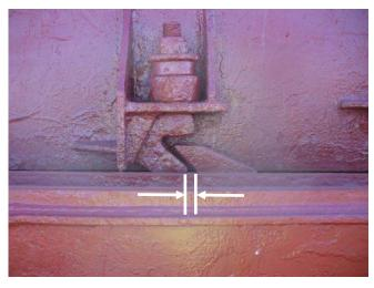
Excessive gap of hatch cover side cleat
