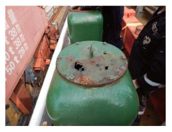
Corrosion holes in air pipe head
