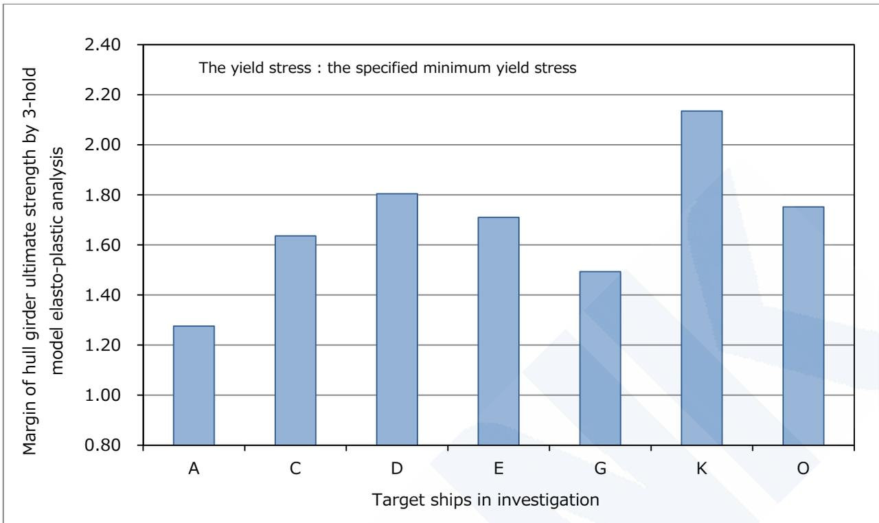
Fig. 4-3 Margin of hull girder ultimate strength calculated by 3-hold model elasto-plastic analysis in consideration of effect of the lateral loads (Margin against the wave-induced vertical bending moment specified in IACS UR S11)
