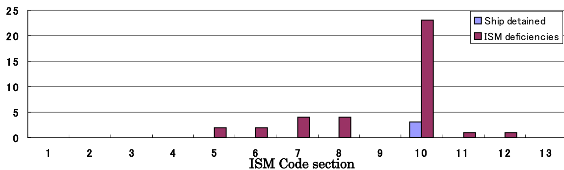
Fig. 2.4.3 ISM Deficiencies that caused a ship's detention, sorted by ISM Code section
