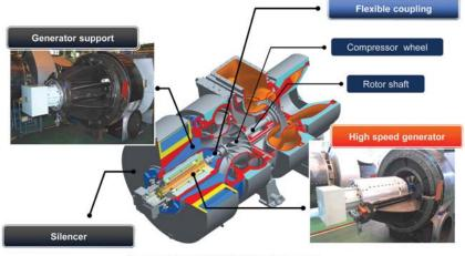
Cross section of MET83MAG turbocharger
