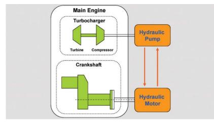
Concept of the THS; Hydraulic pump: Take out excess energy of exhaust gas from the Turbocharger Hydraulic motor: Assists rotation of crank shaft with recovered hydraulic power
