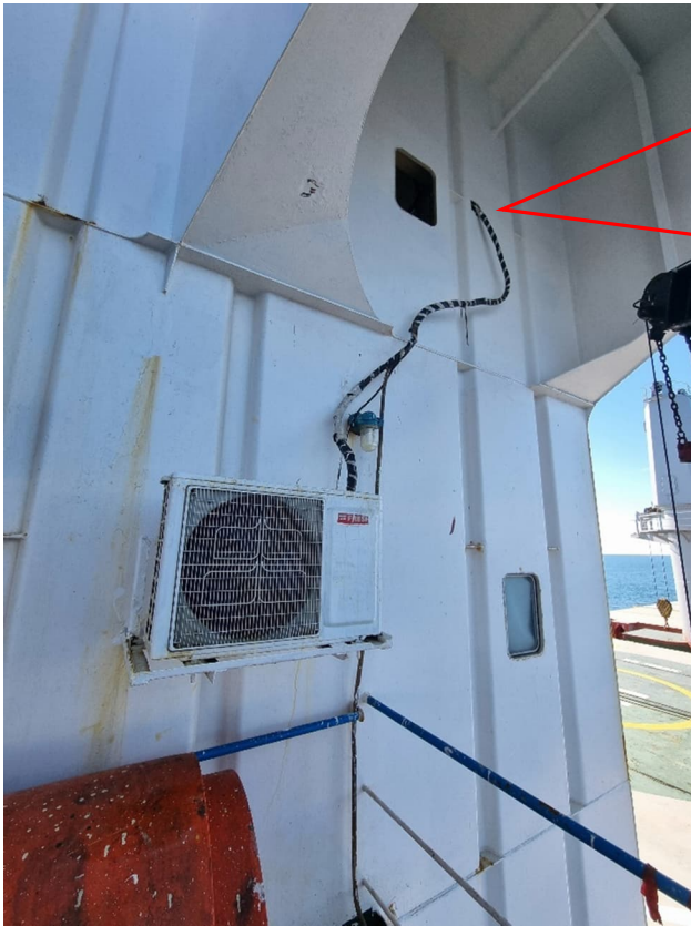
Unauthorized cable installation and penetration through bulkhead
