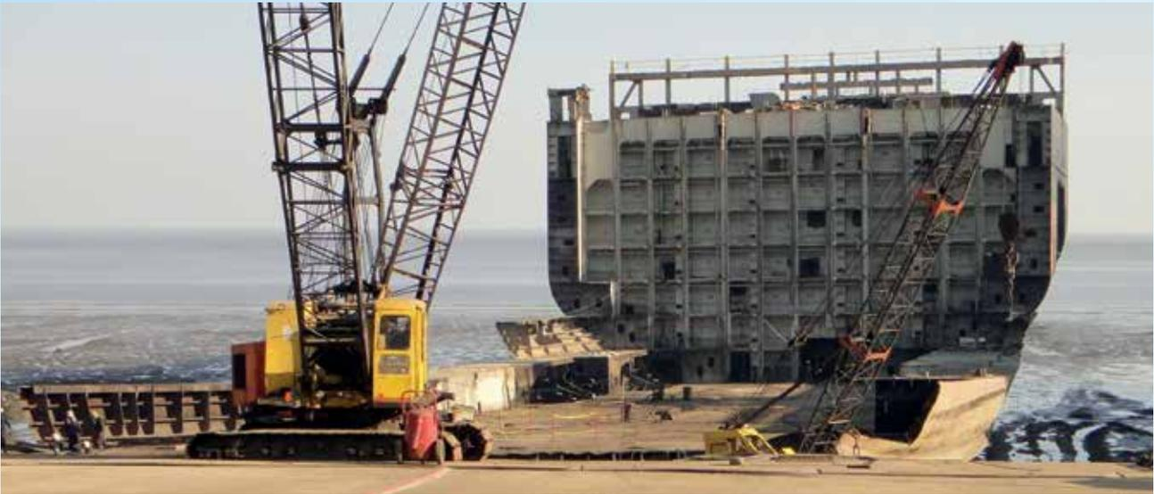
Around 700 of the estimated 45,000 ocean-going ships in the world are taken out of service every year. Their valuable steel - over 80% of a ship's lightweight value - is an available resource that can be recycled. The machinery and equipment included in the lightweight value are also resources that can be reused.
