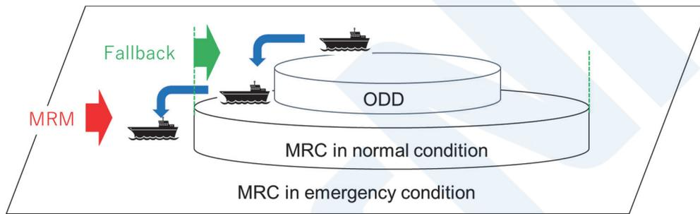
Figure 4 Relationship between ODD, Fallback, MRC, and MRM
