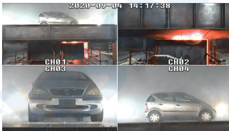
Figure 6 Photograph of vehicle fire experiment: Condition of vertical arrangement
