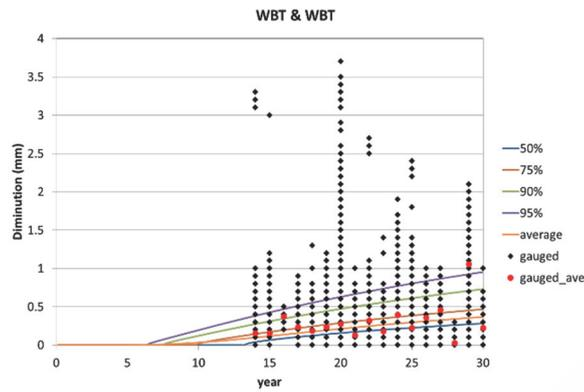
Fig. 3 Estimated corrosion diminution of members of which both sides are exposed to ballast environments
