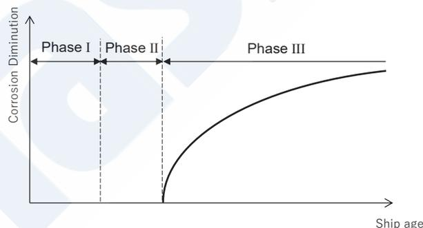
Fig. 1 Consecutive processes of corrosion generation and progress
