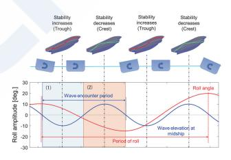
Fig. 2 Development of parametric rolling
