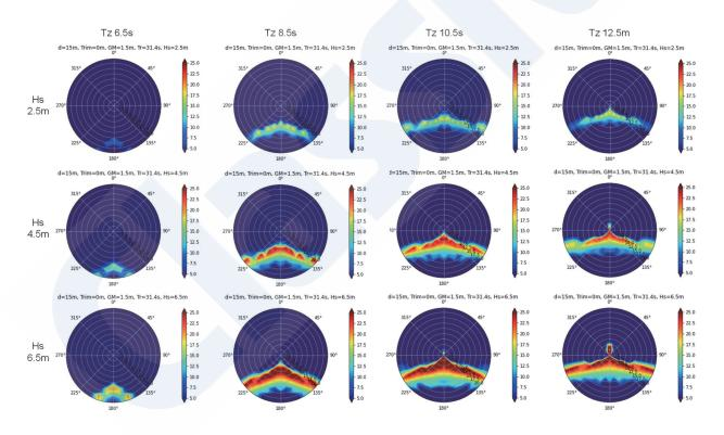
Fig. 7 Examples of polar charts for various significant wave heights and zero-crossing mean wave periods for GM = 1.5 m(Zero-crossing mean wave period  $T_Z$ : 6.5 s, 8.5 s, 10.5s, 12.5 s / Significant wave height  $H_S$ : 2.5 m, 4.5 m, 6.5 m)
