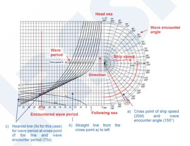
Fig. 3 Determination of the wave period (Source: Notice from Japanese Gov. (MLIT)<sup>14)</sup> based on MSC.1/Circ.1228<sup>13)</sup>)
