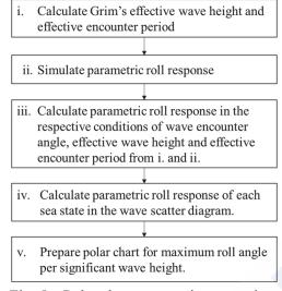
Fig. 5 Polar chart preparation procedure
