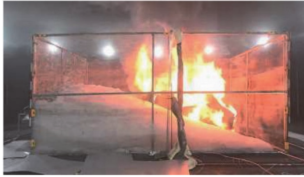
Fig. 8 Condition of BEV covered with foam
