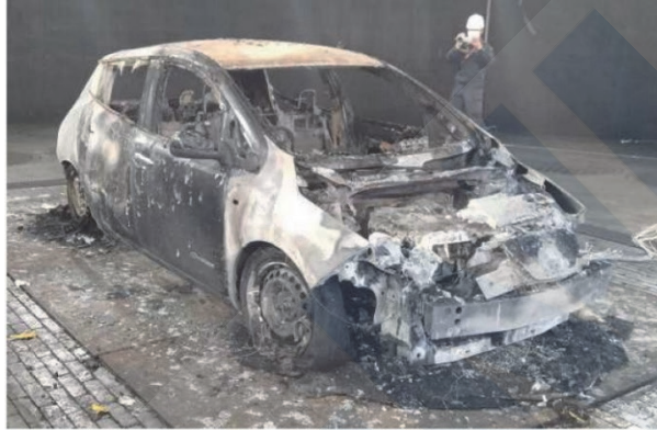
Fig. 9 BEV when wire gauze was removed after the fire
