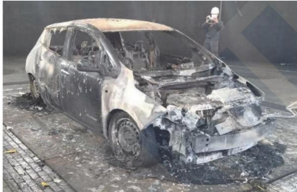
Fig. 9 BEV when wire gauze was removed after the fire
