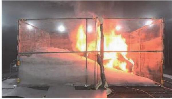
Fig. 8 Condition of BEV covered with foam
