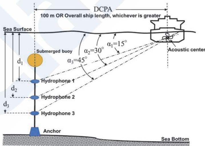
Fig. 1 Example of arrangement of bottom-mounted hydrophones
