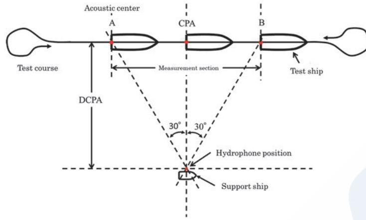
Fig. 2 Measurement configuration(test course and other matters)
