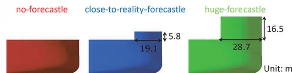
Fig. 8 Side view with assumed forecastle shape model based on BC-10
