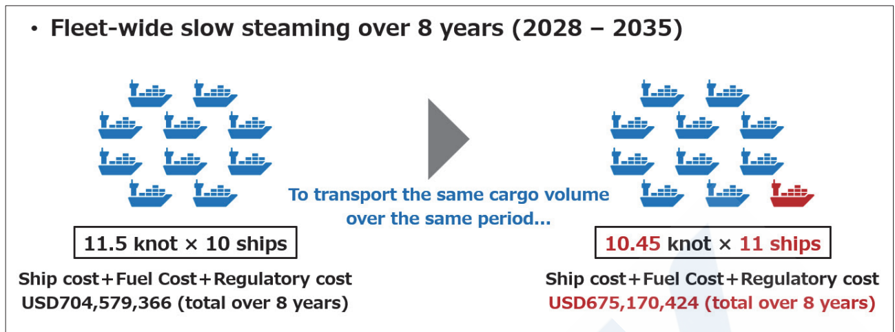
Fig. 9 Cost reduction effect of slow steaming for an entire fleet
