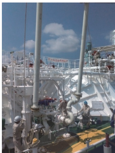
Fig. 4 Loading arm connection during LPG loading (sign indicates loading of flammable hazardous material)
